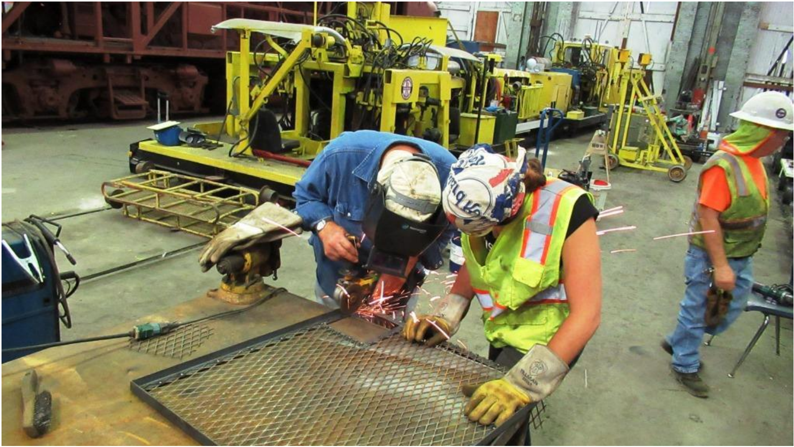
Cliff and Samantha work on the forming a door in the security shield for the ride-on spiker (behind them)
